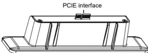
Insert the wireless module into the wireless module slot at the bottom of the device. The wireless module is hot-pluggable.
